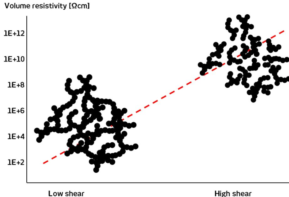
High shear forces often lead to breakage in carbon black network. This results in higher resistance of the moulded parts.
