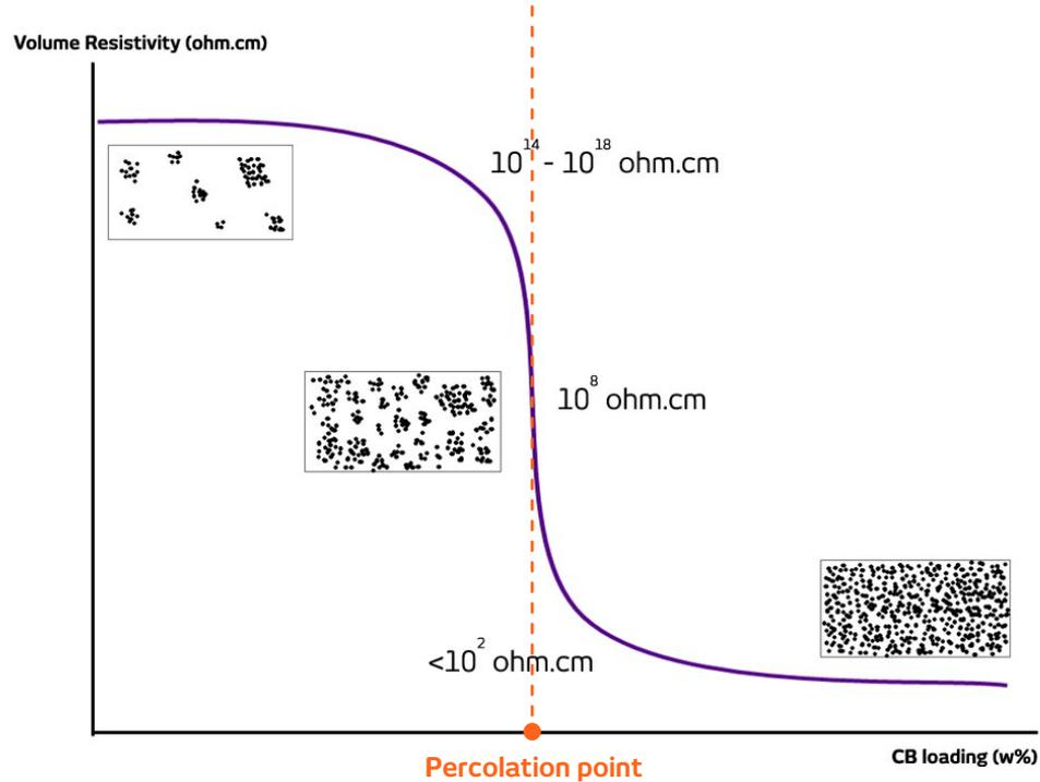
Percolation describes the contact between carbon black particles. At certain carbon black loading level the carbon black particles lose the direct contact between each other and the resistance increases dramatically. This point is called percolation point. Over the percolation point, the change in conductivity is very fast.
